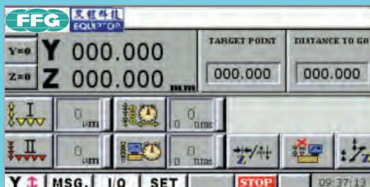
Downfeed ( Rough grinding, Finish grinding, Sparkout setting ) Minimum Display Unit: Y axis 0.001mm / Z axis 0.001mm
