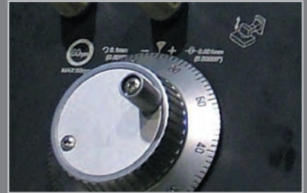
Manual Pulse Generator for Y axis, Z axis by x1 \mu\text{m} / x2 \mu\text{m} / x4 \mu\text{m}
